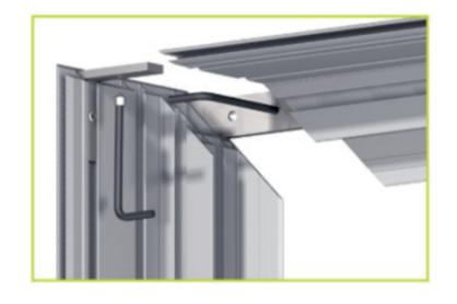
6. REMOVE STAGE WEIGHT, REMOVE TAPE, PLACE THE RETURN FRAME ON THE FLOOR IN A SAFE MANNER, REPEAT THAT ON ALL PARTS 1/4 DEPENDING ON THE WALL SIZE, NOW REMOVE THE SUPPORT BARS USING THE LARGER ALAN KEY PROVIDED, ONCE ALL ARE REMOVED, LAY THE FRAME DOWN AND START LOOSENING BUT NOT REMOVING THE SCREWS ON ONE SIDE OF THE CORNER BRACKET WITH THE SMALLER ALAN KEY PROVIDED, ONCE LOOSENED ON ONE SIDE ONLY, THE FRAMES WILL COME APART LEAVING THE CORNER BRACKET IN PLACE ON ONE OF THE FRAMES.
